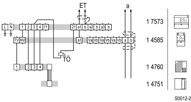
**Circuit diagram:** floor line (ET) to main bus (a).
