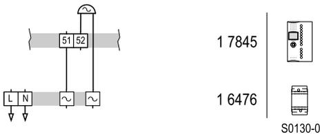
**Circuit diagram:** actuate an external signal encoder via a call interface relay.
