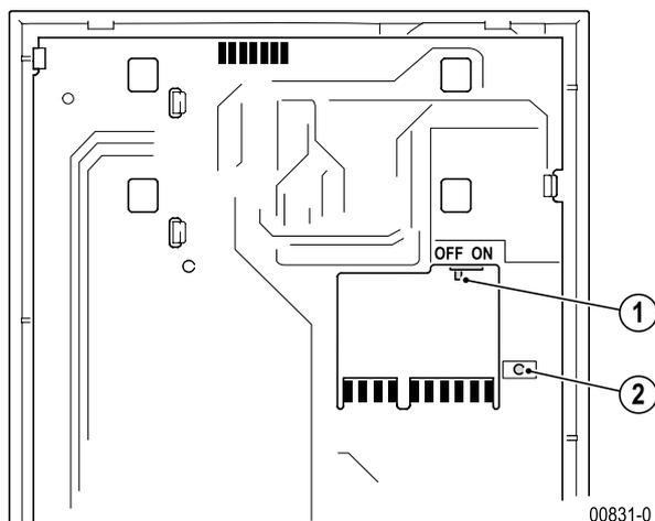
1. DIP switch for activating the terminal resistor (factory setting: OFF)
