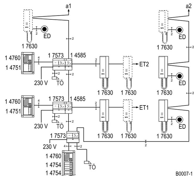
**Block diagram:** multi-family and office building with separate floor access door stations.
