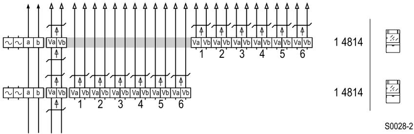
Circuit diagram: Cascading with 2 line switches.
