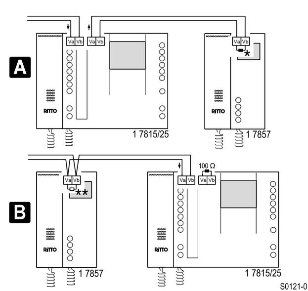
**Circuit diagram:** terminal resistor for mixed systems.
