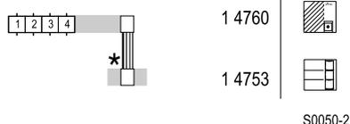
The wire of the bus connector in the door station marked red must be attached to the pin labelled "red" on the board. As a result, the door station modules are numbered identically. The wire marked red is identified in the respective circuit diagram by a "\*".
