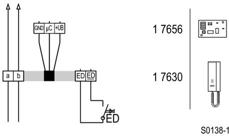
**Circuit diagram:** connection to indoor telephone 1 7630.
