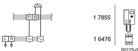
**Circuit diagram:** actuate an external signal encoder via a call interface relay.
