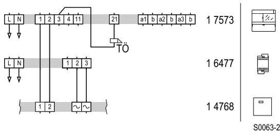
**Circuit diagram:**access module connection as standalone unit.
