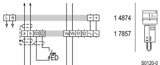
**Circuit diagram:** connection with decentralised power supply.
