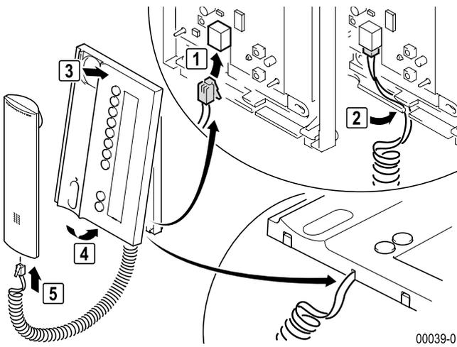
**Concealed and cavity wall installation**
