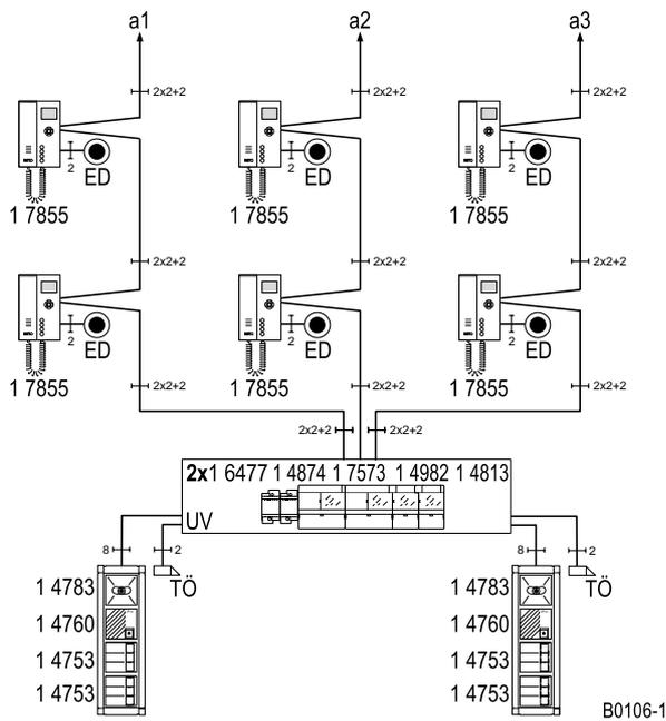
**Block diagram:** multi-family residence with three main bus lines and 2 door stations (central power feed).
