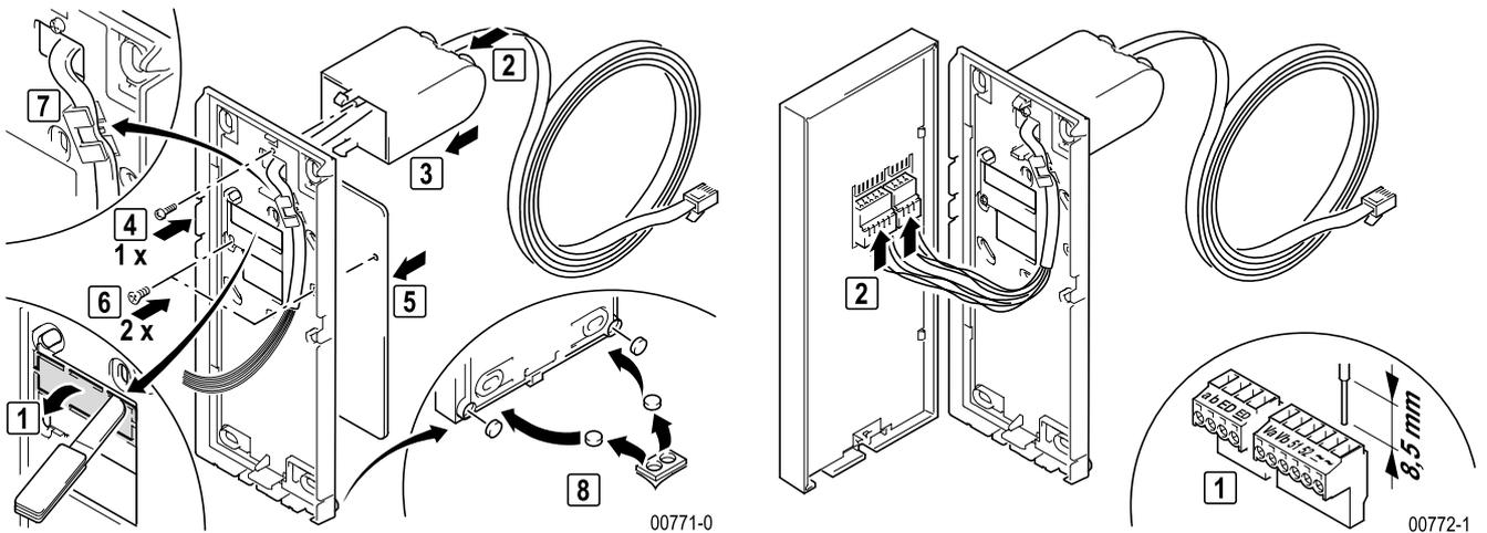
► Connect and install IAE box as shown in table.
