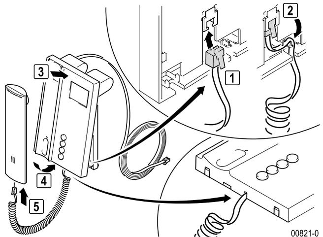
► Connect and install IAE box as shown in the table.
