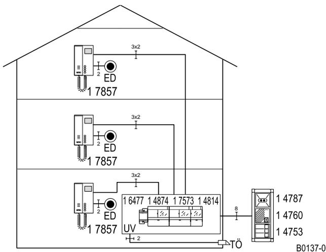
**Block diagram:** video-door intercom system with line switch.
