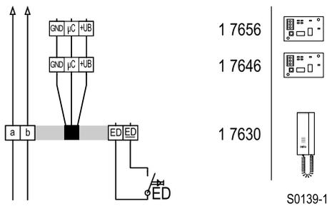
**Circuit diagram:** connection to indoor telephone 1 7630 with call interface relay 1 7646.
