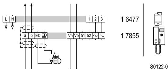
**Circuit diagram:** connection with decentralised power supply.
