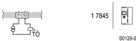
**Circuit diagram:** trigger automatic door opening using the apartment button.
