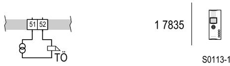
**Circuit diagram:** trigger automatic door opening using the apartment button.
