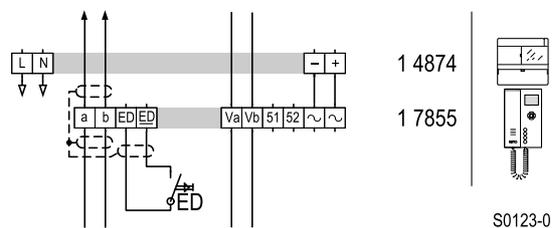
**Circuit diagram:** connection with central power supply.
