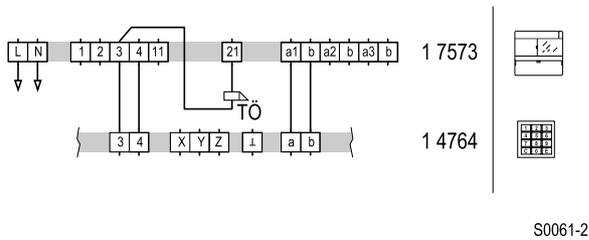
**Circuit diagram:** coding module connection as standalone unit.
