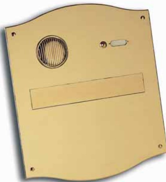
ART. 7111 Frontale sagomato per cassetta postale ad un pulsante e griglia citofonica Shaped front for letter-box with one pushbutton and grid for intercom mm 380x445 Scatola incasso complete with embedding box mm 370x360x270
