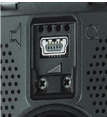
Mini-USB connection and loudspeaker/microphone volume adjustment
